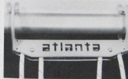
1. Roller Reefing Claw — allows mainsail to be matched to wind conditions
