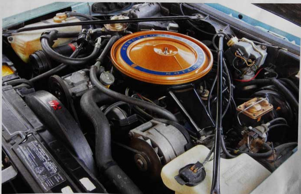
The Seville's only engine in 1976 was the Oldsmobile 350-cu.in. V-8, fitted with electronic fuel injection. Rated at 180hp, the Seville was the first American car designed to have an EFI V-8 engine. Not only did it offer more power than a comparable carbureted engine, it had cleaner emissions and eliminated rough-idle issues.
